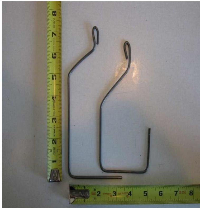
You will want to cover the bare metal with something to keep the gun from getting scratched and slipping off the bar. I used a Plastisol base tool dip but duct tape, electrical tape or a small rubber hose slipped over the metal will work.
