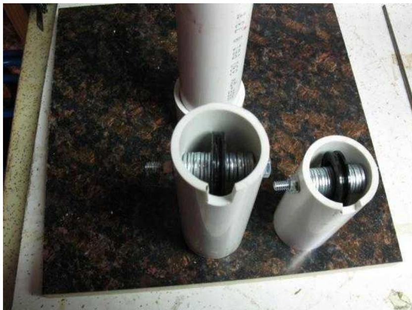
Cut a notch no more than 1/4" wide and 1/2" in for the line to run through. This will be used to trap the fender washer and keep the pistol hook from being pulled into the pulley, derailing the line.
