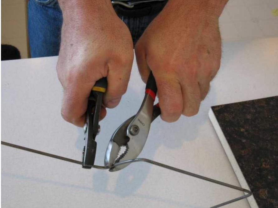
The sizes shown in the picture work well for us but are by no means mandatory. I recommend that you do not put an up turned "hook" on the horizontal bar that the pistol rests on. It serves no real purpose and snags the gun if the shooter does not lift the gun all the way up.
